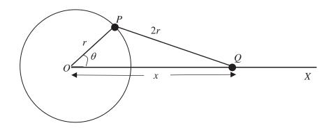
The diagram shows a mechanism for converting rotational motion into linear motion. The point P is on the circumference of a disc of fixed radius r which can rotate about a fixed point O. The point O can only move on the line OX, and O are connected by a rod of length O and the disc rotates, the point O is made to slide along OX. At time O and O is O and the distance O is O is O.
